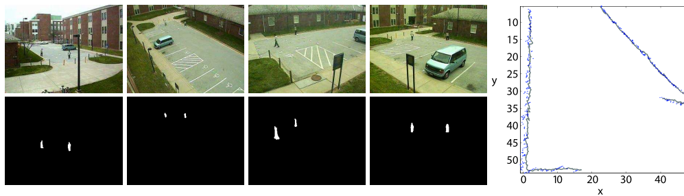
Fig. 10. Tracking results on a video sequence of 300 frames. Results are obtained using only 1/5 the bandwidth required of traditional central servers. (Left) The first two rows show sample images and background subtraction results using the compressive measurements, respectively. The background subtracted blobs are used to detect target location on the ground plane. (Right) The detected points using CS (blue dots) as well as the detected points using full images (black). The distances are in meters. Figure courtesy of [44].
