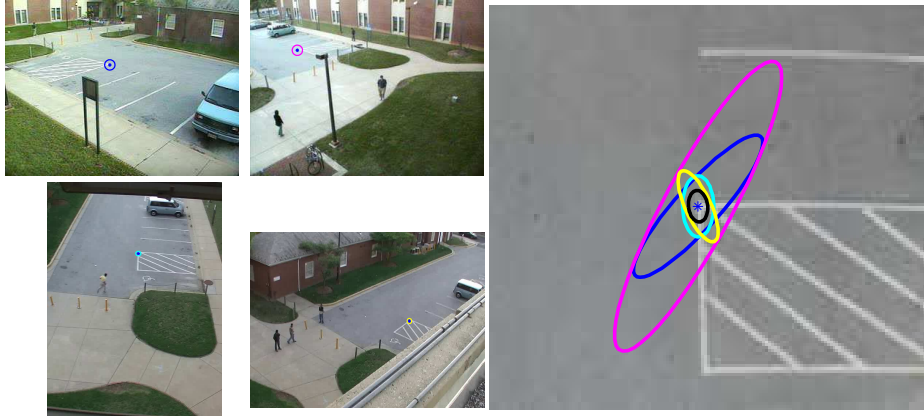
Fig. 4. Variance Ellipses are shown for the individual image planes. The corresponding color coded ellipse on the ground plane shows the covariance when transformed to the ground plane. The ellipse in black (on the ground plane) depicts the variance of the minimum variance estimator. Note that this estimate performs better than the individual estimates. Figure courtesy of [5].
