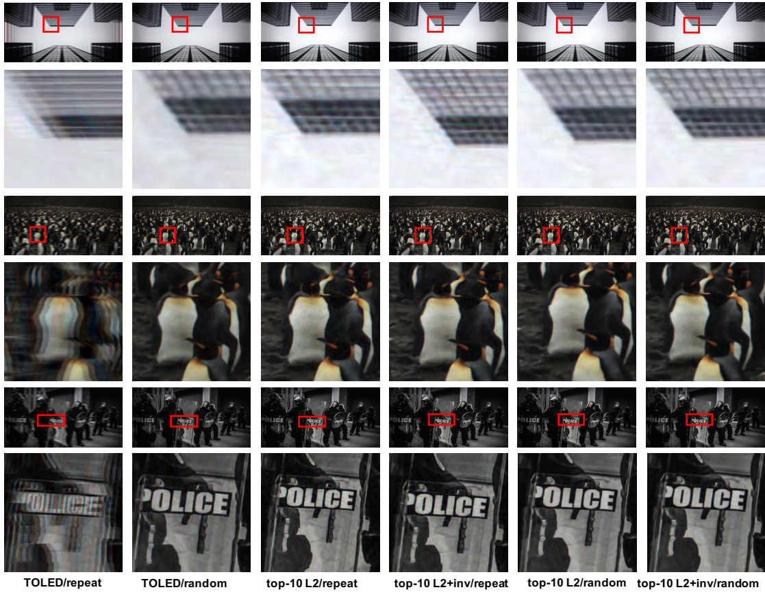
Figure 3.13: Simulated results under six different displays. The display masks have a pixel density of 150 DPI and we compare performance under noise level SNR=28. We show three scenes and their zoom-in patch for comparison.
