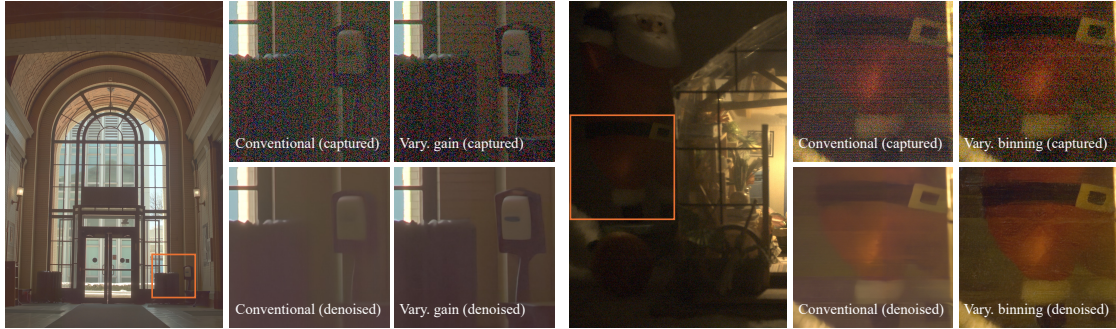
Figure 5.9: Effect of transformer-based restoration networks. Left example is captured by Nikon Z5 and right BFS-U3-200S6C. The upper row shows the captured image after demosaicking and gamma correction, and the lower row shows the above images denoised by Restormer [Zamir et al. , 2022]. (Left) Compared to conventional sensor, the proposed spatially-varying gain recovers much more object details in the dark lighting; (Right) Compared to conventional, spatially-varying binning retains better contrast and recovers sharper contours.
