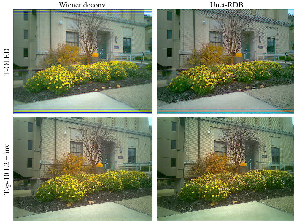
Figure 3.24: Comparison of deblurring methods. We compare Wiener deconvolution with UNet-RDB on an outdoor scene captured under conventional T-OLED and our optimized pattern.
