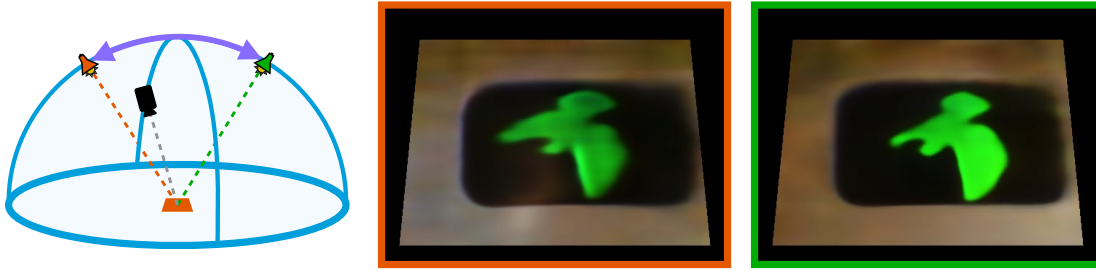
Figure 7.5: Fixed viewpoint renderings. We render the captured Hologram with a fixed viewpoint while moving the illumination in an arc over the object from right to left (see diagram). Note that the dove’s left wing is more extended when illuminated from the right (orange) and more retracted when illuminated from the left (green). This creates an effect where the dove appears to rotate in space.
