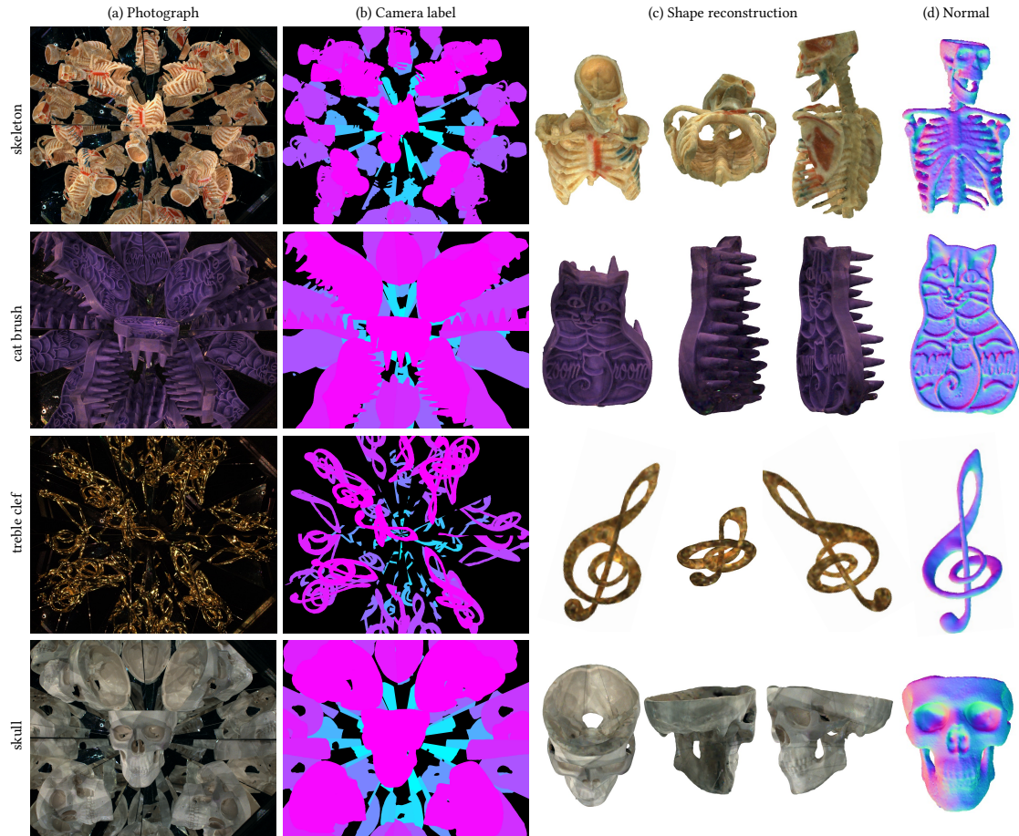
Figure 3.13. Real object scans from our prototype. Reconstructed point clouds and full-surround videos are available on the project webpage [Ahn et al. , 2021b].
