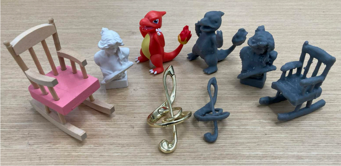
Figure 4.1. 3D printing of shape reconstructions. The proposed neural kaleidoscopic space sculpting can generate replicas of real objects with a range of shapes and reflectances.
