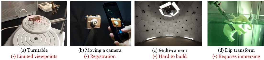
Figure 1.1. Non-kaleidoscopic full-surround 3D reconstruction approaches. (a) Rotating an object constrains viewpoints to lie on a plane perpendicular to the rotation axis. (b) Moving a single camera requires the registration for estimating the camera pose. (c) Multi-camera systems are generally costly and difficult to build (d) Dip transform [Aberman et al. , 2017]—a technique that dips the object into a fluid at multiple orientations and reconstructs the shape from liquid displacements—requires immersing the object in the fluid.
