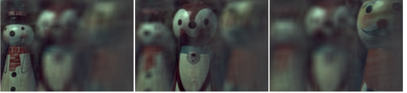
Fig. 1. Lensless focal stack . We show images reconstructed at three different depths using our proposed SweepCam technique, which is a lensless camera with a programmable mask.
