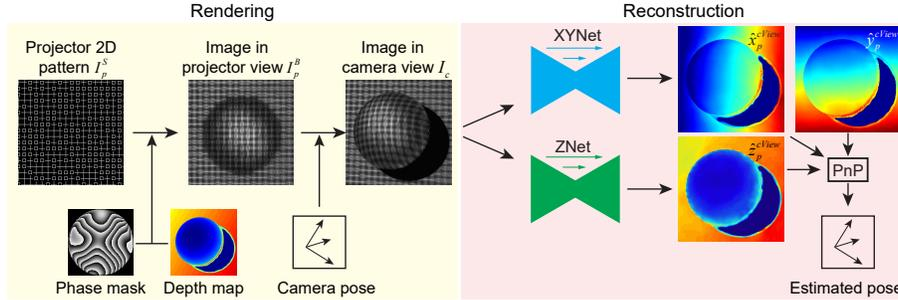
**Fig. 2.** System pipeline. (Left) The forward rendering part builds a physics-based model to simulate the captured camera image for any 3D scene and camera pose. (Right) From the single-shot image  $I_c$ , we first predict the 3D location in the projector coordinate. We then estimate the camera pose with a PnP solver. The pipeline is fully-differentiable, and can be trained end-to-end.
