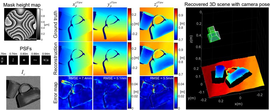
**Fig. 3.** Simulation results. (Left) The learned phase mask and its corresponding PSFs at different depths.  $I_c$  is an example of the input image in simulation. (Center) The output of XYNet and ZNet, containing the 3D map in the projector coordinate. (Right) The estimated point cloud of the scene in the projector coordinate. The estimated camera pose (white) is close to the ground truth (green).
