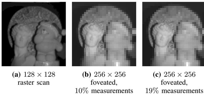
**Fig. 13: Optical wavelet foveation.** Our setup is capable of selectively sampling a region of interest; We show an example here with selectively high resolution sampling over the marble bust. Even with 10% measurements, our method is capable of capturing fine details in the scene.
