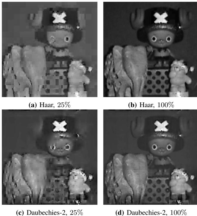
**Fig. 14: Sampling with Daubechies wavelets.** Though Haar wavelets are a popular choice, our setup is capable of capturing any wavelet decomposition. Here we show a comparison with Daubechies wavelets with two filter taps.
