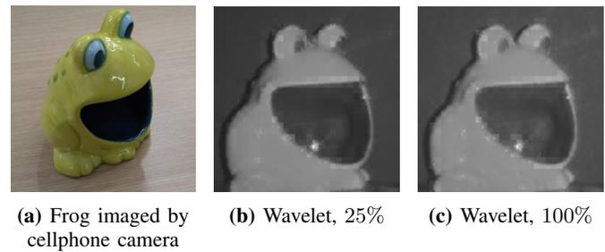
**Fig. 15: Failure due to non-Lambertian BRDF.** When the scene to be imaged is highly specular, active illumination based methods fail to work well. This can be seen from the blocky artifacts on the lips of the ceramic frog.
