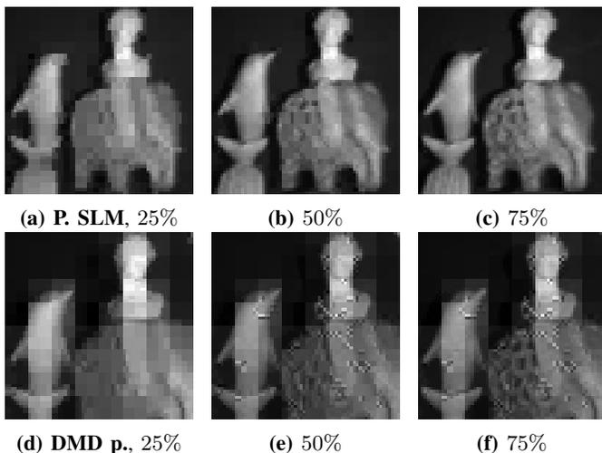
**Fig. 11: DMD projector vs phase SLM.** We captured a  $64 \times 64$  image with a laser projector as well as our prototype to compare the advantages of concentrating light. While the images look similar at low sampling rates, adaptive sensing with DMD adds high frequency artifacts at higher sampling rates, a direct consequence of reduced signal energy.
