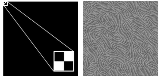
**Fig. 6: Design of phase pattern.** We use Iterative Fourier Transform (IFT) to design phase masks. (a) shows positive part of a diagonal wavelet basis and (b) shows the obtained phase mask. Since wavelet bases of a given scale are simple translations of each other, we generate a single pattern and add an appropriate phase ramp to obtain its translated versions.
