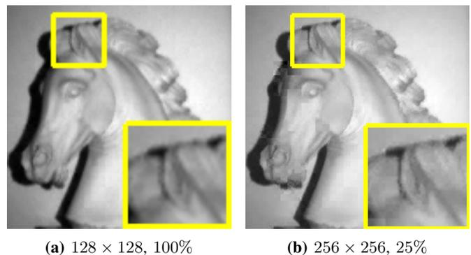
**Fig. 12: Advantages at higher resolution.** Images are sparser as resolution increases, which works in favor of adaptive wavelet-tree parsing. We show an example scene comprising of a horse bust sampled at  $128 \times 128$  as well as at  $256 \times 256$  with same number of measurements. Despite a  $2 \times$  increase in resolution, we achieve finer spatial details without an increase in measurements.
