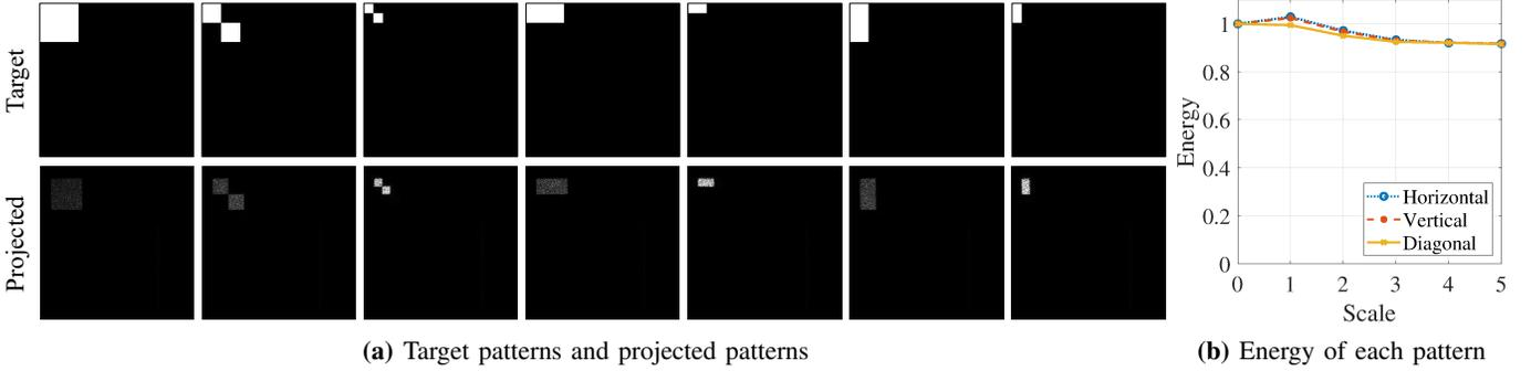
**Fig. 7: Energy vs. scale.** A phase SLM forms patterns by redistributing light, and hence the energy stays constant, independent of shape or scale of pattern. (a) shows target and projected patterns for some Haar wavelet patterns. Note how the intensity in smaller wavelet patterns is higher. (b) shows energy of each pattern as a function of spatial scale, which is almost constant.
