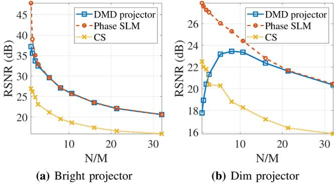
**Fig. 4: Comparison of various imaging techniques.** The plots above show accuracy vs compression for the cameraman image when imaged with a (a) bright and (b) dim projector. We observe using a phase SLM provides significant gains when operating with sources that are not bright.
