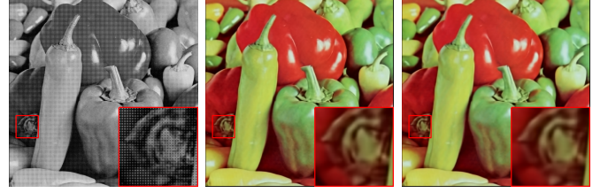
Fig. 1: Left to right: Bayer image, image reconstructed using OMP, and image reconstructed using the proposed method. While OMP takes 16 minutes, the proposed method takes only 1.5 minutes with little loss in reconstruction quality.
