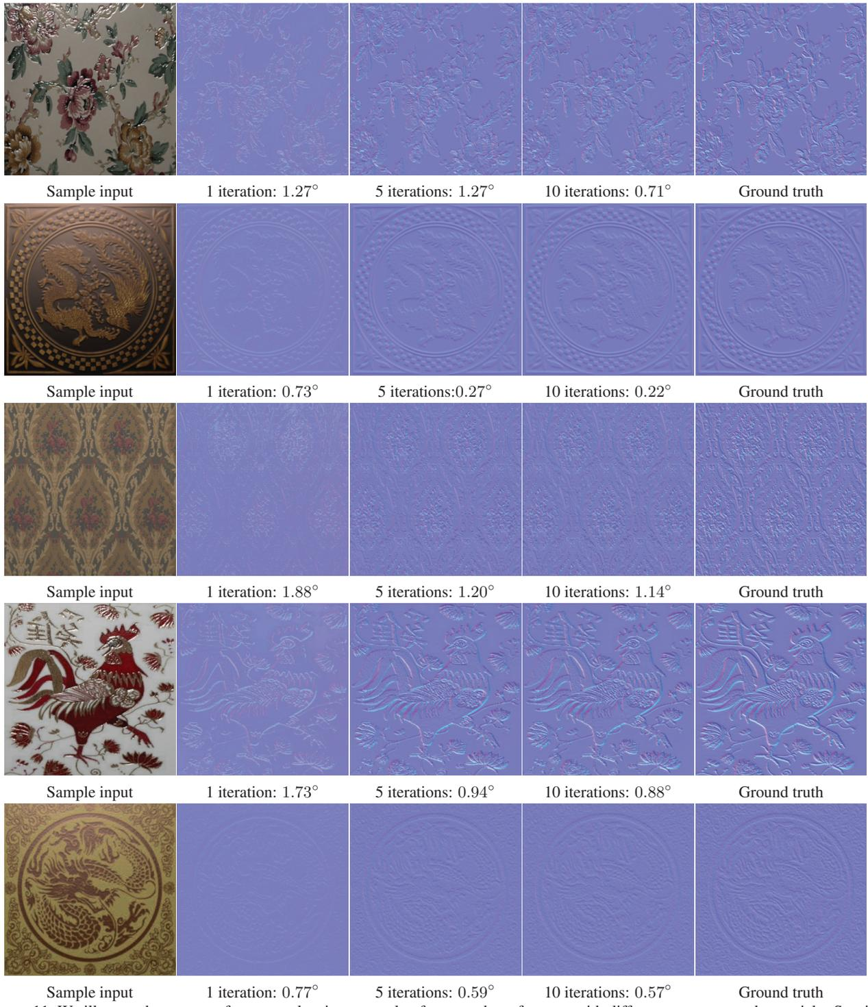
Figure 11. We illustrate how our surface normal estimates evolve for a number of scenes with different geometry and materials. Starting from flat surfaces, our method refines the normals so that over the course of 10 iterations they converge to results that have a mean angular error of only 0.73° to 1.14°.
