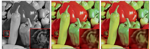
Fig. 1: Left to right: Bayer image, image reconstructed using OMP, and image reconstructed using our proposed method. While OMP takes 16 minutes, our proposed method takes only 1.5 minutes, a speed-up of 10\times .
