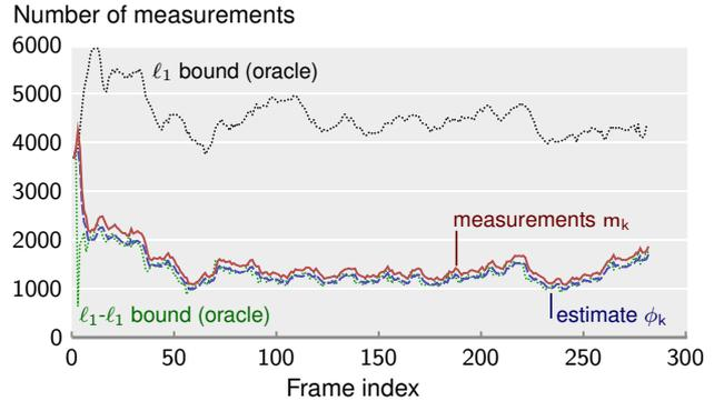
**Fig. 2.** Number of measurements  $m_k$ , estimate  $\phi_k$ , and right-hand side (5) for  $x[k]$  per frame. It also shows the bound for standard  $\ell_1$  minimization [23].
