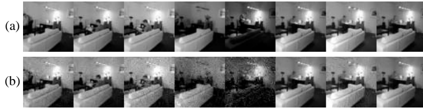
Figure 4: SpaRCS recovery results on a 64 \times 64 \times 234 video sequence. The video sequence is reshaped into an N_1 \times N_2 matrix with N_1 = 64^2 and N_2 = 234 . (a) Ground truth for several frames. (b) Recovered frames. The recovery SNR is 23.9 dB at the measurement ratio of p/(N_1 N_2) = 0.33 . The recovery is accurate in spite of the changing illumination conditions.
