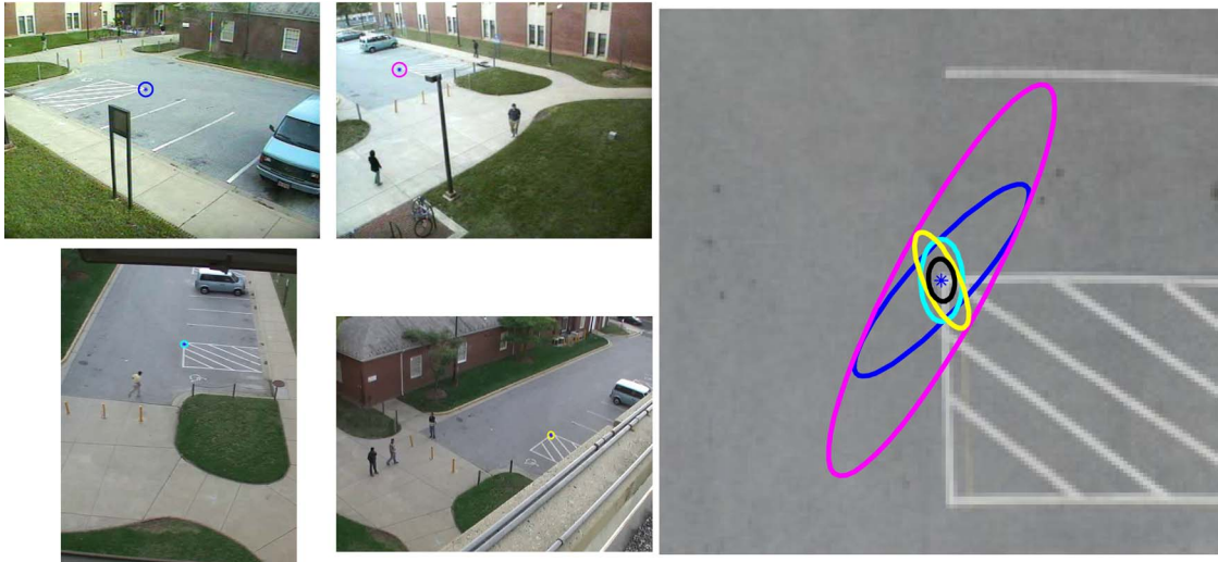
Fig. 5. Variance ellipses are shown for the individual image planes. The corresponding color-coded ellipse on the ground plane shows the covariance when transformed to the ground plane. The ellipse in black (on the ground plane) depicts the variance of the minimum variance estimator. Note that this estimate performs better than the individual estimates.
